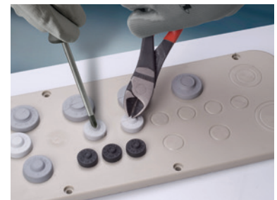
Make a small hole into the membrane using a screwdriver or cut the top of the cone using side cutters.
