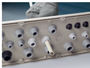
(Back side) Pull the cable or tube back for some 20 mm to lock it.
