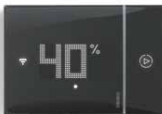
Display the set room temperature and humidity
