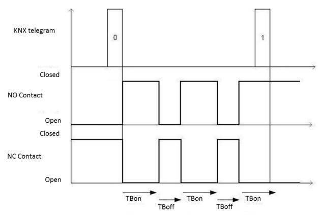
If you select **value "1"**, then when the device receives a telegram from the BUS with a logic value equal to "1", it switches the relay to the status  $\rightarrow$  NO contact closed/NC contact open, and begins the activation time count; At the end of the activation time, the device deactivates the load (NO contact open/NC contact closed) for a period of time equal to the deactivation time, and then reactivates the load and restarts the process. See the following figure for more information.
