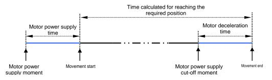
NOTE: the times set for the "Motor start time" and "Motor deceleration time" parameters are only used to calculate the time required to reach a certain intermediate percentage position (following a specific command, or following the reproduction of a position associated with a scene or prior to a status). They are not used for any movements carried out via the **Ch.y/z** - **Movement** object.
