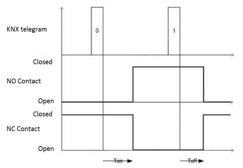
Selecting **value "1"**, when the device receives a telegram from the BUS with a logic value equal to "1", after the set activation delay time (Ton) has passed it switches the relay to the status  $\rightarrow$  NO contact closed/NC contact open; Vice versa, when the logic value "0" is received, the device waits for the deactivation delay time (Toff) before switching the contact to  $\rightarrow$  NO contact open/NC contact closed. See figure below.
