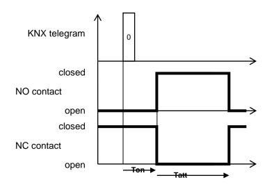
Selecting **"1" value**, when the device receives a telegram from the BUS with a logic value equal to "1", after the set activation delay time (Ton) has passed it switches the relay to the status  $\rightarrow$  NO contact closed/NC contact open. See figure below.
