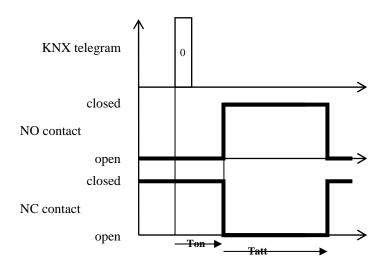
Selecting **value "1"**, when the device receives a telegram from the BUS with a logic value equal to "1", after the set activation delay time (Ton) has passed it switches the relay to the status  $\rightarrow$  NO contact closed/NC contact open. See figure below.
