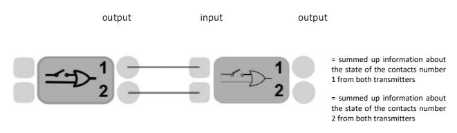
The system also allows for connection of signals of different types, performing for this purpose an automatic conversion before summing up.
