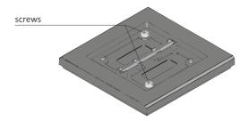
3 Disconnect the button stand from the frame and electronics.
