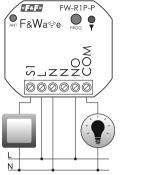
control input triggered by level L
