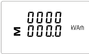
Total reactive energy in kVArh
