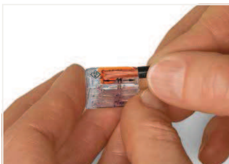
Strip conductor to 11 mm (0.43 inch).
