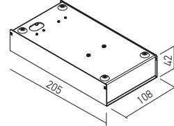
Box for installing of the drivers for the systems of XCLICK S SURFACE and XCLICK M SURFACE profiles with maximum powers of 200W.
