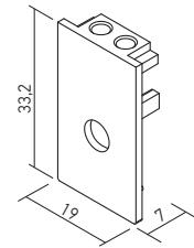
End cap for the recessed or surface profiles of the XCLICK S system. Provided with central access hole for power supply cable.
