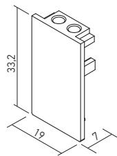
End cap for the recessed or surface profiles of the XCLICK S system.
