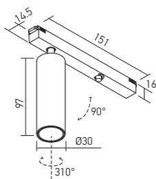
Adjustable and dimmable (PWM) mini projectors for installation in the profiles of XCLICK S RECESSED and XCLICK S SURFACE systems, equipped with power LED, mechanical fastening system.
