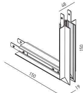
Structural element with recessed mounting, for the mechanical connection of two linear profiles at 90°, in different mounting planes (external angle), equipped with electrical circuit for 48V DC. It is mounted in plasterboard dropped ceilings or walls, trimless installing.
