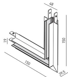
Structural element with recessed mounting, for the mechanical connection of two linear profiles at 90°, in the same mounting plane, equipped with electrical circuit for 48V DC. It is mounted in plasterboard dropped ceilings or walls, trimless installing.
