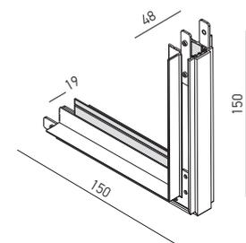
Structural element with recessed mounting, for the mechanical connection of two linear profiles at 90°, in different mounting planes (internal angle), equipped with electrical circuit for 48V DC. It is mounted in plasterboard dropped ceilings or walls, trimless installing.
