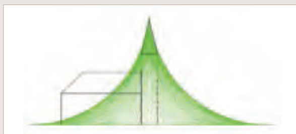
Protected area in accordance with EN 62305, standard III protected level (sphere radius R=45 m)
