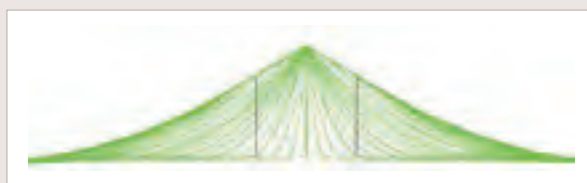
Protected area in accordance with EN 62305, standard III protected level (sphere radius R=45 m)
