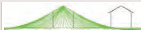
Protected area in accordance with EN 62305, standard III protected level (sphere radius R=45 m)
