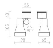
Outdoor spotlight with a reflector that can tilt by loosening a screw between the reflector and the base.
