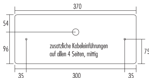
Bohrabstände PF Wand/Decke / drilling holes PF wall/ceiling
