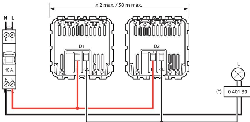
(\*) For some electronic loads, the installation of a compensator Cat. No. 0 401 39 is required.
