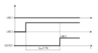
6.3 Maximum switching time upon connection of Line 1 with Line 2 present
