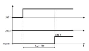
6.2 Maximum switching time upon connection of Line2 with Line1 absent 1.15s
