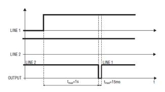
${\bf 6.4}$  Maximum switching time upon disconnection of Line1 with Line2 present
