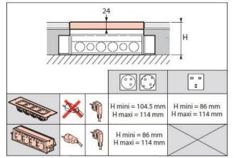
Box cross-section with height specification for horizontal support installation
