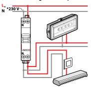
The branch can be joined in the electric cabinet, on the switch or in a junction box.
