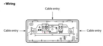
REMOTE CONTROL - Connection terminals: no polarity with the Legrand remote control Cat. No. 0 039 00/01. Terminal capacity:  $2 \times 2.5 \text{ mm}^2$ .
