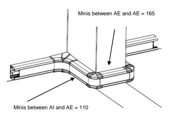
Mini dimension in mm to be respected allowing the installation of angle inter/exter: (in the case of a skirting of post for example)
