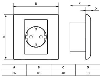
Distance of installation hole: 60.3 mm
