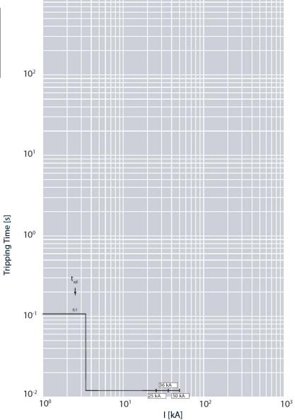
$I_{cu}$  = 36-50 kA  $I_{max}$  = 250A 4 P  $U_{e}$  = 415Vac (IEC/EN 60947-2)
