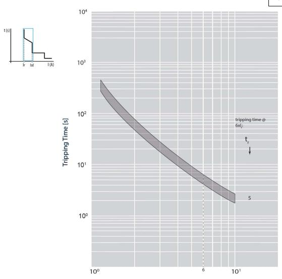
$\label{eq:I_cu} I/I_{_{\Gamma}}$   $I_{\text{cu}} = 36\text{-}50 \text{ kA} \quad I_{\text{max}} = 250 \text{A} \quad 4 \text{ P} \quad U_{\text{e}} = 415 \text{Vac} \quad \textit{(IEC/EN 60947-2)}$
