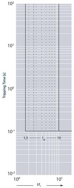
$I_{cu}$  = 36-50 kA  $I_{max}$  = 250A 4 P  $U_{e}$  = 415Vac (IEC/EN 60947-2)
