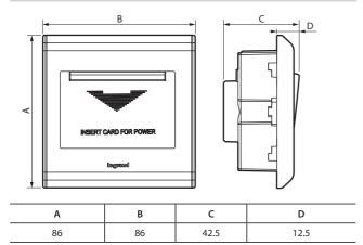
Distance of installation hole: 60.3 mm
