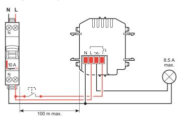
Pressing the auxiliary control allows the load to be switched on or off manually. If no action is performed on the control, the detector will cut off the related load at the end of the time delay or when the Daylight setpoint is reached.
