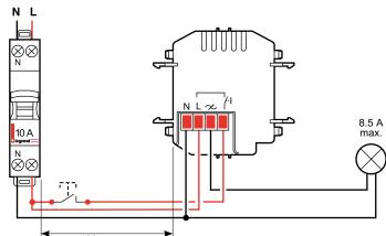
Pressing the auxiliamasontrol allows the load to be switched on or off manually. If no action is performed on the control, the detector will cut off the related load at the end of the time delay or when the Daylight setpoint is reached.
