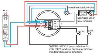
Two channels (switch & dim) with a single manual control for dimming
