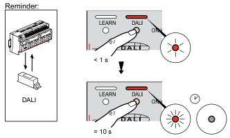
DALI ballast: total lighting of all loads, then gradual dimming and switching off of the loads in a random order.
