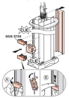
A - put the normaclip on the body and clip it B - push it down
