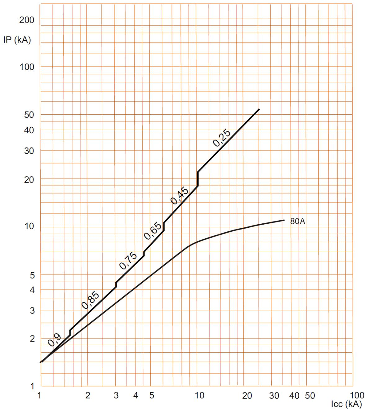
. I<sub>cc</sub> = Square value of symmetric component of the short circuit current ( kA ).
