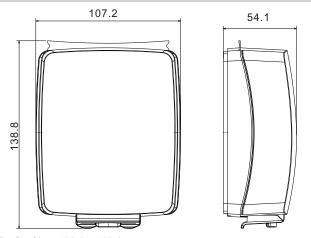
Profile Size: 138.8×107.2mm Distance of installation hole: 60.3 mm
