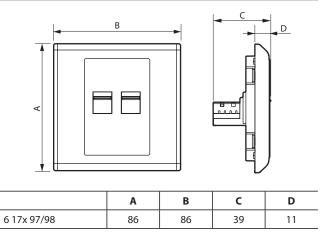
Distance of installation hole: 60.3 mm
