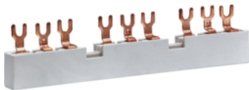
Bareta 3P pt. 3 disjunctori motor 63A 10mm 2
