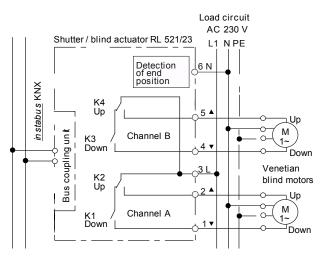
figure 1. Example of operation
