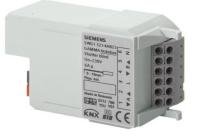
The RL 521/23 shutter / blind actuator is a KNX device with two relay output channels. The device is installed in an AP 118 Control Module Box or an AP 641 room control box. The bus is connected via a bus terminal block. The actuator electronics are supplied via the bus voltage. The RL 521/23 may be used to control blinds, shutters, awnings, windows, or doors.
