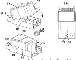
figure 3: Mounting of an RL module
