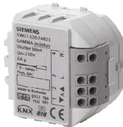
The RS 520/23 shutter / blind actuator is a KNX device with one relay output. The device is installed in an AP 118 Control Module Box or an AP 641 Room Control Box. The bus is connected via a bus terminal block. The actuator electronics are supplied via the bus voltage.
