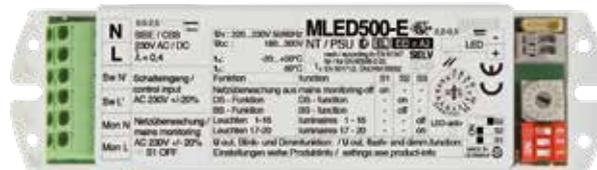
The MLED500-E is an electronic switching power supply with integrated individual light monitoring, light management function, mains monitoring, dimmer and flashing functions. It supplies LED illuminants with a max. output of 8W. The MLED500-E is suitable for use with emergency lighting systems of type: **multiControl plus, midiControl plus, miniControl plus, microControl plus and myControl plus.**
