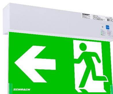
Self-contained emergency luminaire according to EN 60598-1, EN 60598-2-22, ISO 7010 and EN 1838 for wall- or ceiling mounting with single or double sided labeling. Suitable for maintained and non-maintained operation. Pictogram set (left, right, up down and white) included. The emergency light function can be blocked via a potential-free contact at terminals f+/f-.
