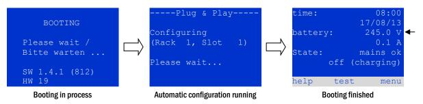
Figure 20: Boot process (left, middle) and status message (right).
