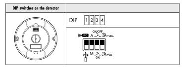
Individual adjustments can easily be made by remote control or manually by means of adjusting elements selected by operating the selector switch DIP 1 (see illustration).
