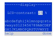
Figure 61: Setting the LCD-contrast
