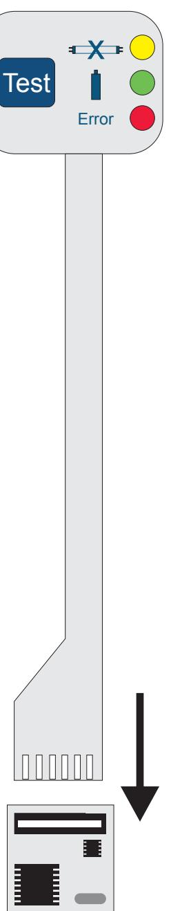
The SelfControl-Module is a quartz controlled monitoring unit for self-contained luminaires, which automatically performs weekly functional tests and annual duration tests.
