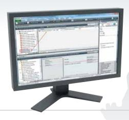
ETS software for the configuration of KNX devices
