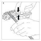
6. Use the front punching part for punching center holes for screw mounting
