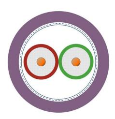
Conductor bare copper conductor, solid copper,
