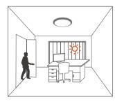
The light keeps off during daytime even when movement is detected. (Ambient lux triggered on 100% by the level is above preset daylight threshold)
