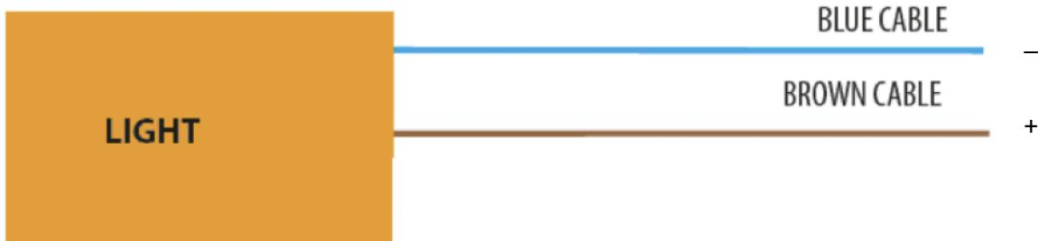
Please connect the cables according to the drawings above.
