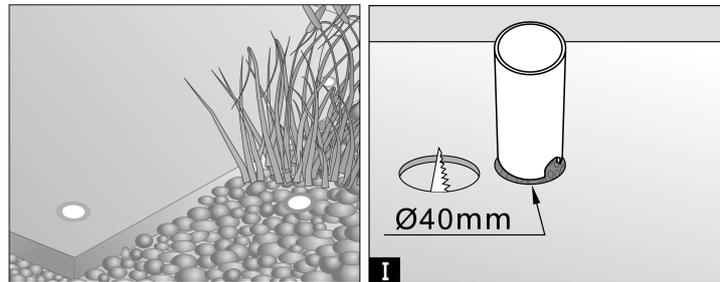
Drill a hole in the desired location, in order to install the recessed spot, with a diameter of 40mm at the top. So be careful not to have too much or not enough drilling.
