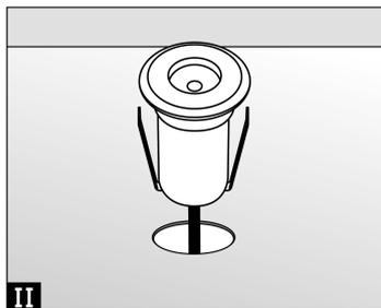
Insert your spot into the drilled spot, taking care not to trap the wiring.
