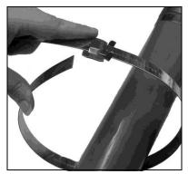
1. Band may be used from bulk roll as this completely eliminates waste of band. Slide buckle on band as shown, bringing end of band around object to be clamped and again through buckle. NOTE: The tension screw thread should be lubricated regularly.
