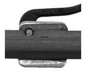
1. Remove gripper. Align gripper pin hole with notch in tool frame. Using a punch and hammer, punch pin out of slide block.
