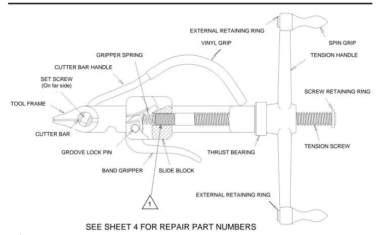
. To assist in removing threaded parts, apply heat (softens locking compound).
