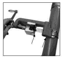
3. Place band in opening of tool nose and gripper block. Move into slot as far as possible, to avoid buckle sliding into tool nose. Tighten band clamp by turning the tension handle clockwise while holding band gripper tight against band. NOTE: The spring load of the band gripper is not intended to secure and prevent band from slipping during tension process.
