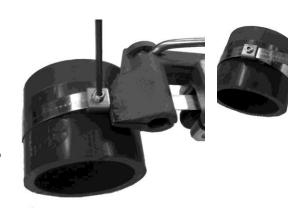
2. After tension is applied, insert set screw in Scru-Lokt buckle and tighten. To permit taking up Scru-Lokt clamp, or to re-use, a 3 inch (7.5 cm) stub should be left so that tool will be able to re-grip band later.
