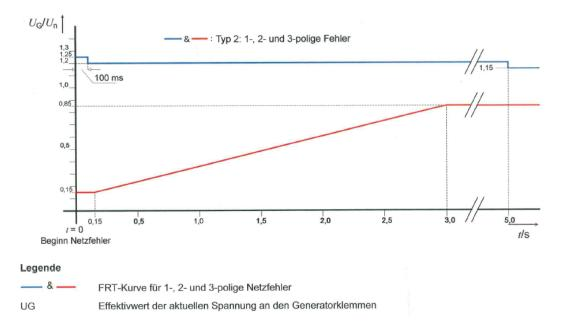
(FRT profile according to VDE-AR-N 4105:2018 Type2- converter and others)
