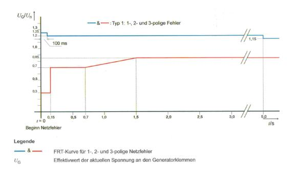
(FRT profile according to VDE-AR-N 4105:2018 Type1- synchronous generators only)
