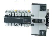
ATyS d M devices are 2 pole or 4 pole transfer switches that are remotely controlled using volt-free contacts from an external controller. They are modular products with positive break indication. They are intended for use in low voltage power supply systems where a brief interruption of the load supply is acceptable during transfer.
