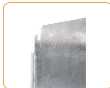
Mounting plate is made of galvanized steel sheet with a thickness of 2 mm. Mounting plate is fixed to the body with screws M8x25 mm. Depending on the size, special foldings of the plate edge are made for better stiffness.
